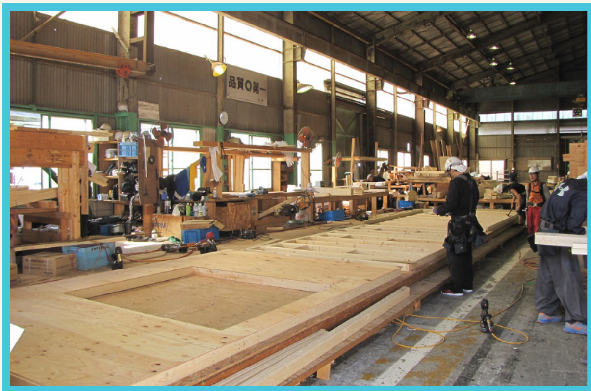
Figure 5: 2-D panel being built in a factory.
